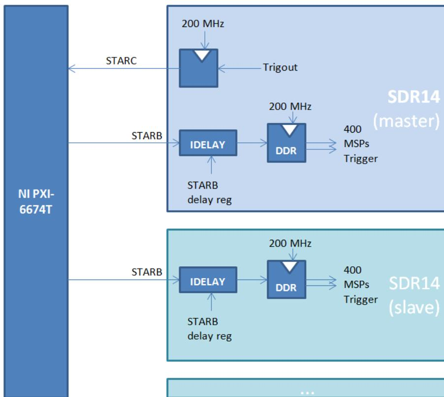
This setup has been verified to have deterministic relative phase between the output waveforms across multiple startups and is already successfully used in customer applications.
