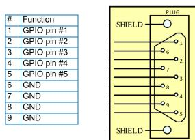
Figure 4: GPIO connector.
