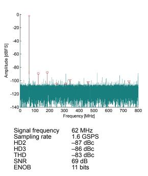
Figure 3: Typical spectrum at 62 MHz.
