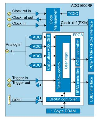
Figure 1: Block diagram.
