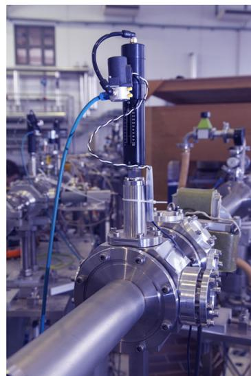
Figure 42: A time-of-flight mass spectrometer.
