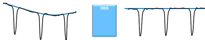
Figure 7: When enabled, DBS will constantly monitor the baseline and correct for variations.
