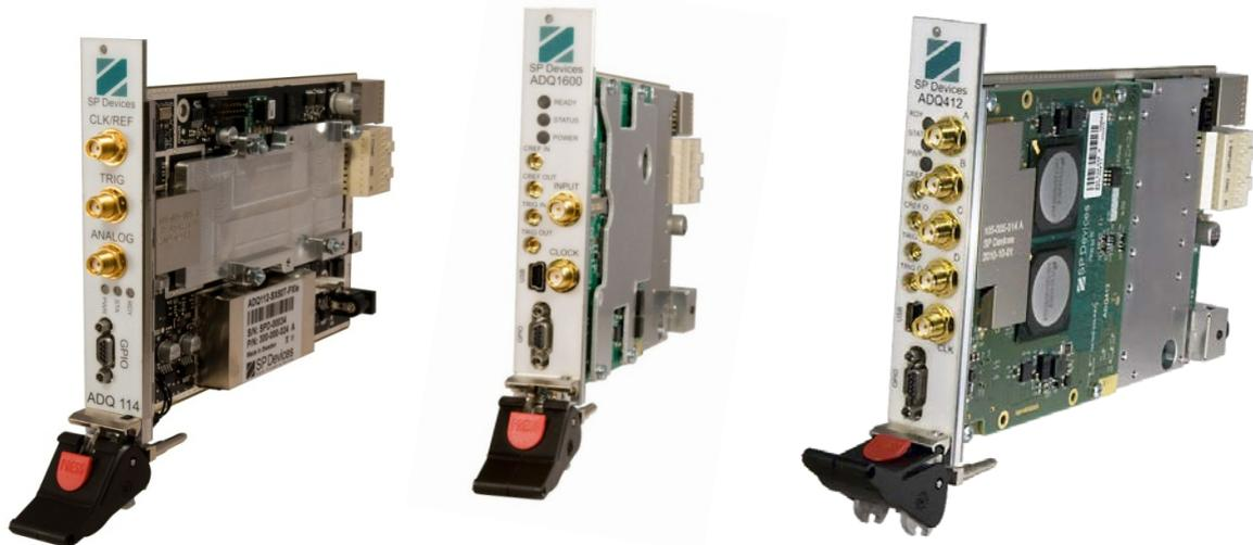
Figure 4: Three digitizer product models of SP Devices. To the left, an ADQ114 in a PXIe format. The single analog input is sampled at 800 MS/s and the resolution is 14 bits. This is enabled by two time-interleaved Texas Instruments ADS5474 ADCs and an embedded real-time implementation of the mismatch error correction IP-core ADX2 from SP Devices.
