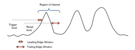
Figure 10: An example of a region of interest, consisting of the region between the start and the end of the pulse, as well as leading and trailing edge windows.
