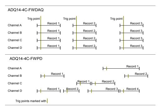
Figure 2: The –FWPD adds dynamic recording, which is illustrated with an ADQ14-4C example.
