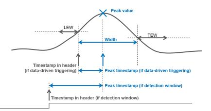
*Figure 36:* The two cases of how the peak timestamp is related to the header timestamp illustrated in the same picture. The detection window (if it exists) is typically triggered by the internal or external global trigger source.
