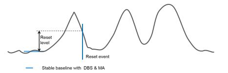
Figure 14: The end of the pulse is the reset event.
