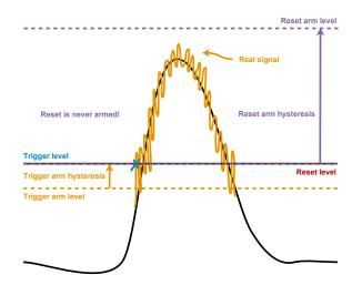
Figure 16: Example of a bad choice of reset arm hysteresis. The reset event will be missed.
