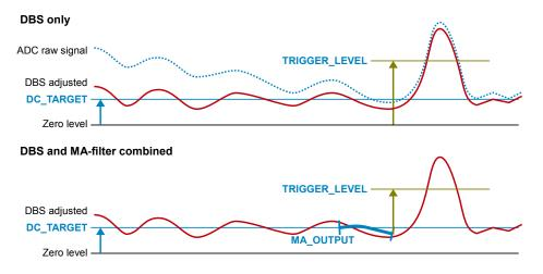
Figure 13: The user-specified trigger\_level is defined differently, depending on if the MA-filter is enabled or not. With a active MA filter in the trigger\_level perspective, dc\_target will be the new zero-level.
