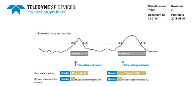
Figure 34: The data-driven level trigger can set the record header timestamp.
