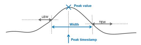
Figure 20: Illustration of the standard analysis metrics peak value, pulse width, and peak timestamp. LEW and TEW is not included in the pulse width.
