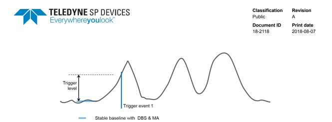
Figure 12: The start of the pulse is the trigger event.
