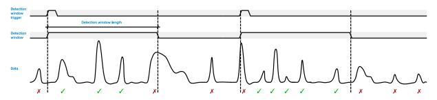
Figure 17: An example of how a detection window is used to mask undesired pulses. Pulses marked with a green check mark are accepted. Pulses marked with a red x-mark are rejected.
