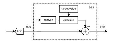
Figure 6: DBS principe of operation. Input data is analyzed and variations are compensated for. The baseline is adjusted to the target value set by the user.
