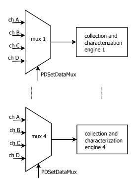
Figure 37: Illustration of collection mode flexibility with the data multiplexers on ADQ14. Any of the four input channels can be connected to any of the characterization engines.
