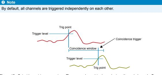
Figure 18: Coincidence trigger overview. The green channel is dependent on the red channel. Green channel triggers are only accepted if the red channel has triggered. Coincidence triggers are only accepted within the Coincidence window.
