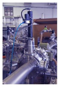
*Figure 42: A time-of-flight mass spectrometer.*
