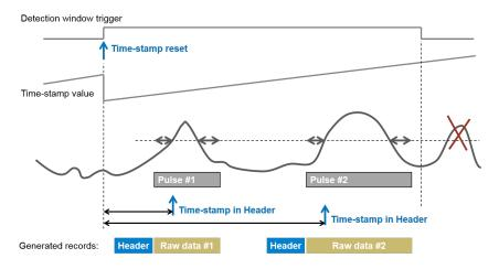
Figure 35: Timestamp example with timestamp reset at start of detection window.
