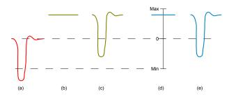
Figure 4: Analog input DC-offset adjustment with margin, to allow for overshoot.
