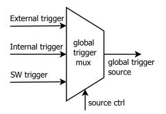
Figure 39: Control of global trigger source.
