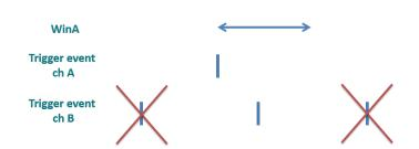
Figure 19: Coincidence window for channel A and exemplitying trigger events on channel B with  $Mask_{BA} = 1$ , that is channel B is dependent on channel A.
