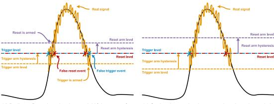
(d) Badly configured arm levels may yield false events from the incorrectly detecting pulses within the signal noise.
