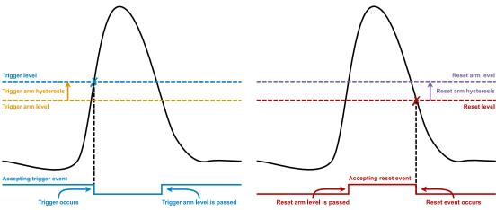
(b) The trigger arm level is determined from the trigger level and the trigger arm hysteresis. The level is used to arm the mechanism generating trigger events.
