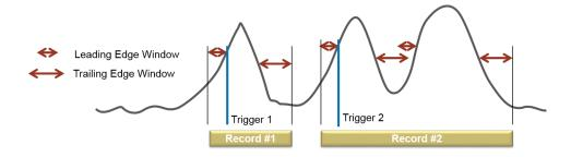
Figure 31: If trailing and leading edges of two pulses overlap, the will end up in the same record as shown for Record #2.
