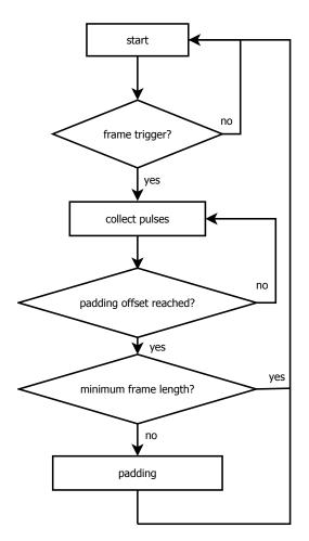
Figure 30: Flow graph of data collection in Mode 3 and Mode 4.
