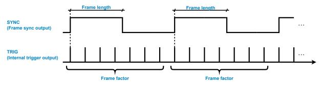
Figure 40: A trigger distribution example with frame factor 7.
