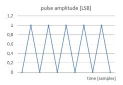
Figure 43: Detectable pulse train with settings for TOF MS.
