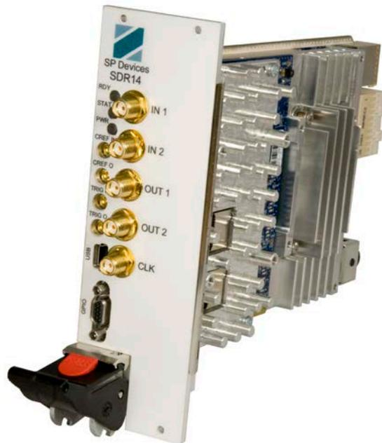
The high-speed SSD (Solid State Disc) recording system is optimized for recording the radar data from the digitizers. The transmission is enabled by the SDR14's standard embedded arbitrary wave form generator. Other required advanced features are channel synchronization and image processing capacity.
