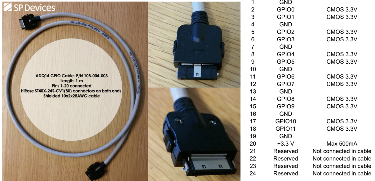
Figure 28: ADQ14 GPIO cable connection (options –GPIO, –VG and–MTCA).
